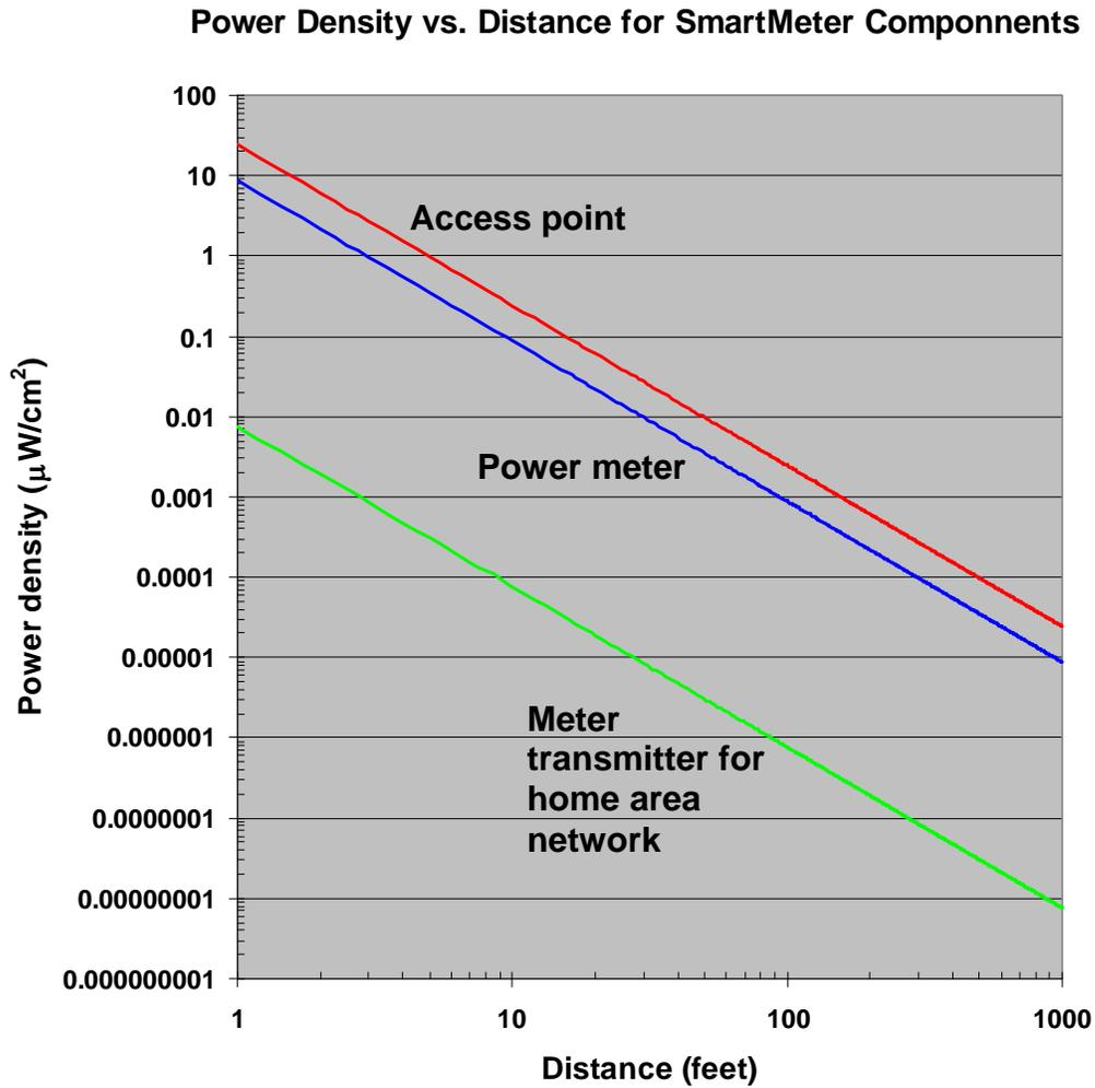
Figure 2. Calculated RF power density vs. distance for the SmartMeter Program Upgrade meters, access points, and internal meter home area network transmitter. Repeater units would produce RF fields greater than the power meter curve and less than the access point curve.
